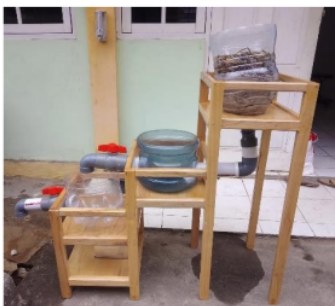
Fig. 18: Prototype of SLW processing system. The methods including filtration, sedimentation and ozonization.
