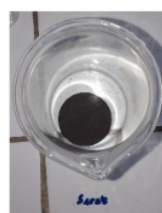
Fig. 7: Fiber-based Ceramics after porosity test.
