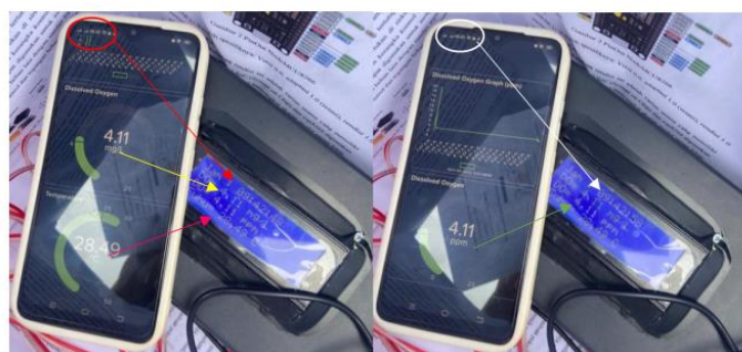
Figure 5. Testing and validating of the IoT-based monitoring system
