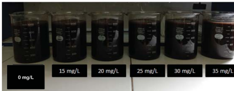
Figure 4. Coal wastewater samples after treated with PAC as coagulant with a dose range of 0-35 mg/L
