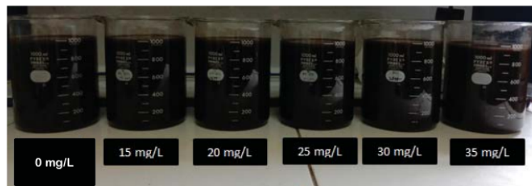
Figure 3. Coal wastewater samples after treated with \text{Al}_2(\text{SO}_4)_3 as coagulant with a dose range of 0-35 mg/L.
