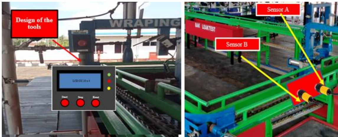
Figure 2. System tool layout planning Monitoring automatic tube counter at SPBE PT Batuah Energi Indonesia
