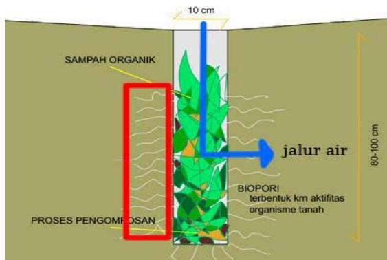
**Gambar. 2** Sketsa Penampang Lubang Resapan Biopori
