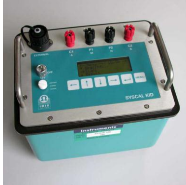
Gambar 19. Resistivity Meter, Syscal Kid Resistivity Meter serial RS232
