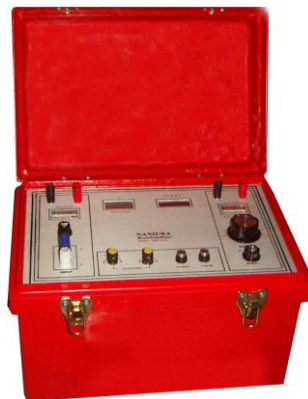
Gambar 7. Instrumen Resistivity Meter, Naniura Model NRD 22 S
