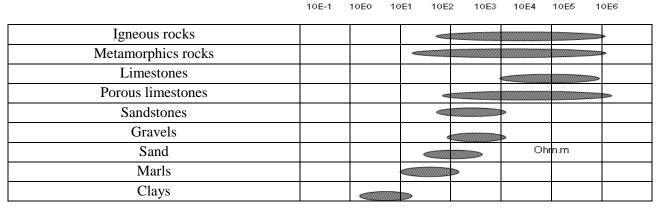
Based on the results of the interpretation of the geoelectrical estimation with the help of a computer and it has been correlated with local geological and hydrogeological data, the resistivity log is obtained at each estimation point as shown in the following table below:
