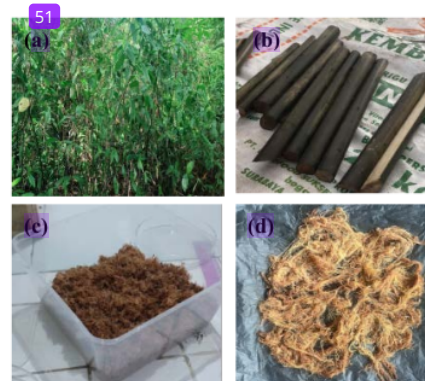
Fig. 1 Mechanism Process of Bemban Fiber: (a) Bemban plant; (b) Bemban stem cut from Bemban plant; (c) Bemban fiber before alkalinization; (d) Bemban after alkalinization
