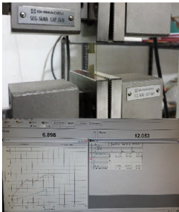
Fig. 12 Tensile loading mechanism and tensile test graphs
