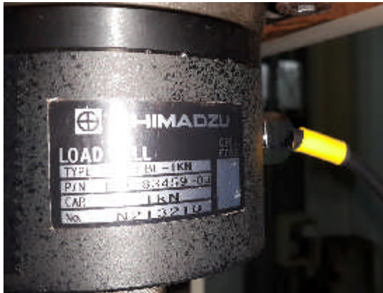
Fig. 10 Load cell were used on fiber tensile testing
