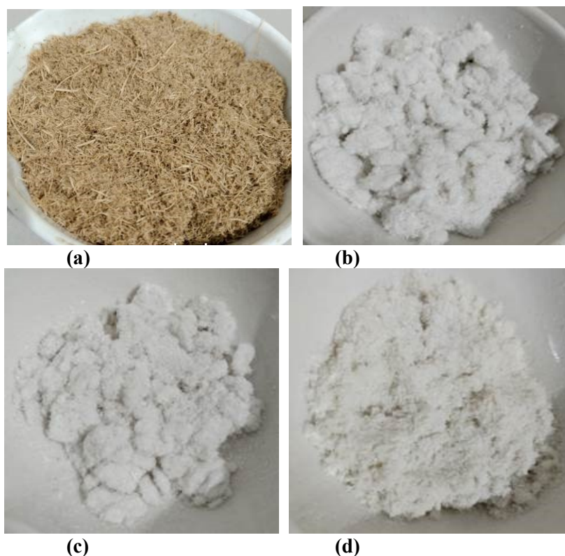
Figure 2. Color appearance a) OPEFB fiber; b) Cellulose of bleaching 2x-delignification; c) Cellulose of bleaching 2x-delignification at temp of 70-80°C; d) Cellulose of delignification-bleaching 2x.
