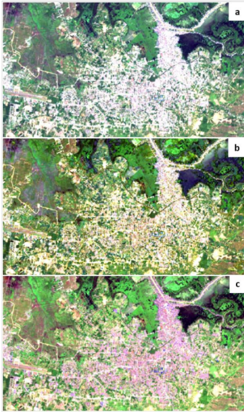
Fig. 6. Urban features on Landsat 8 OLI imagery composite 432, (a) Original TOA imagery, (b) USGS TOC imagery, and (c) Radiometric enhancement imagery using exponential equation without parameter
