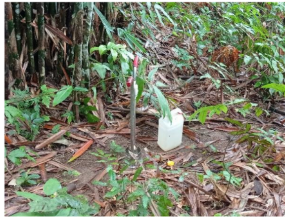
Fig. 1 Infiltration Rate Testing in Datar Ajab Village, Hulu Sungai Tengah District
