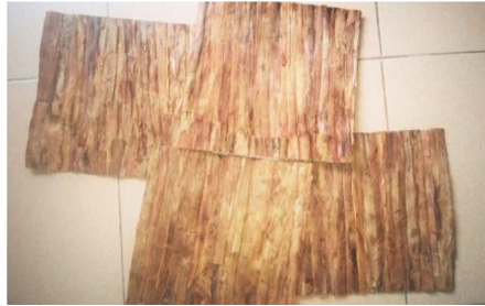
Fig. 4. Results of sewing gelam bark fibers.
