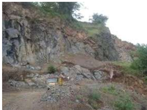
Figure 4. Open Mining as Triggering Factor for Rock Fall
