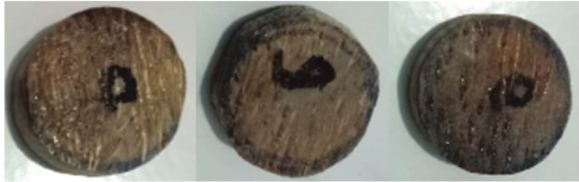
Figure 7: Specimen samples for acoustics test: pH 4, pH 6 and pH 10
