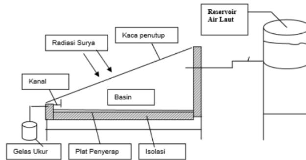
Gambar 2. Bagian-Bagian *Solar Distillation*
