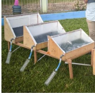
Gambar 1. *Solar Distillation*
