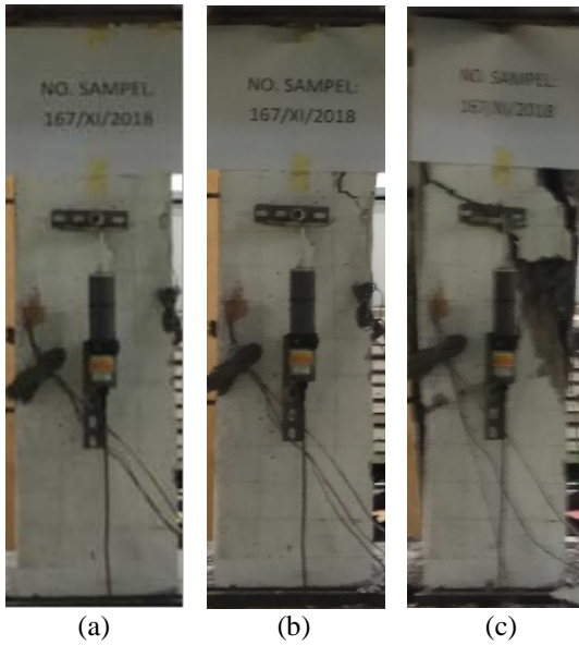
Fig. 13 Failure progress of SPIP specimen during testing. Source: authors
