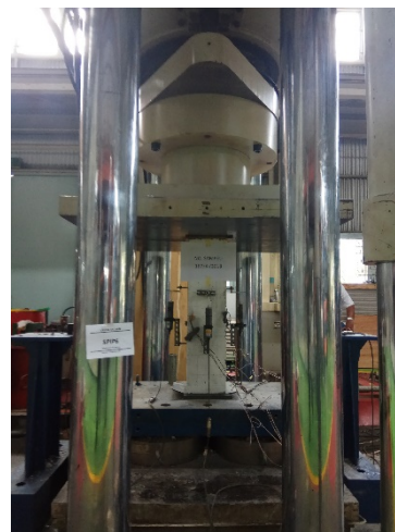
Fig. 2 Photograph of UTM with a specimen ready for testing. Source: authors
