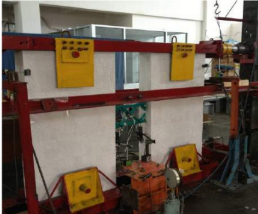
Fig. 3. The coupling beam with shear wall (laboratory specimen)
