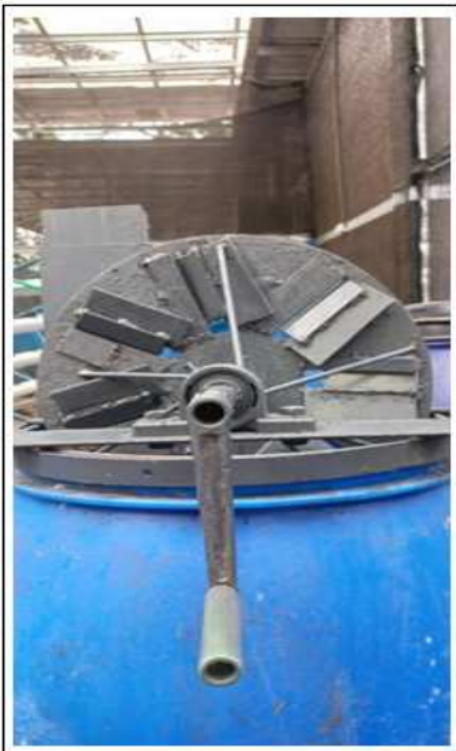
Fig. 4. Compost Bin with a Chopper.
