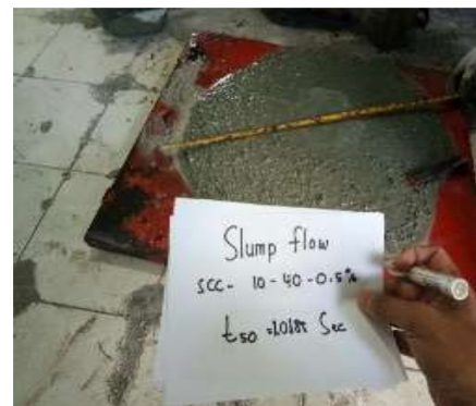
Figure 7. Slump Flow Test (Actual test)
