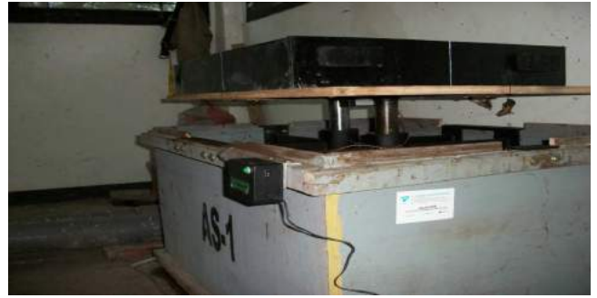
Fig. 3 A laboratory model of stabilized fibrous peat
