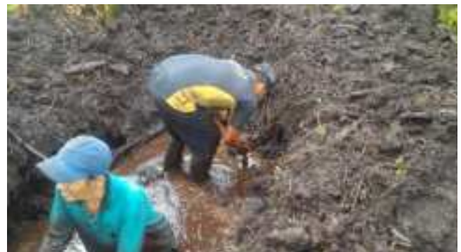
Fig 1. Undisturbed fibrous peat sample taking.
