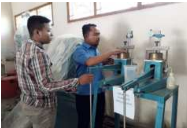
Fig. 7 Consolidation test of fibrous peat
