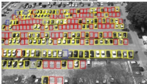
Figure. 11 Misclassification example on cloudy weather condition
