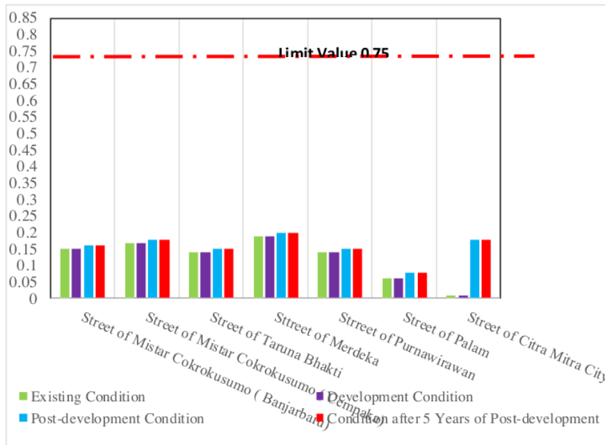
Fig.12: The DS Values of Each Condition towards the Limit Value of Handling
