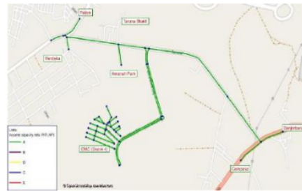
Fig.10: The LOS Simulation and the Amount of the Traffic Flow of the Road Section of Post-development at Peak Hour
