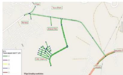
Fig.9: The LOS Simulation and the Amount of the Traffic Flow of the Road Section during the Development at Peak Hour
