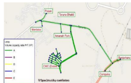
Fig.11: The LOS Simulation and the Amount of the Traffic Flow of the Road Section of the 5-year Post-development at Peak Hour
