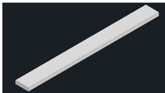
Gambar 2 Desain Standar Objek ASTM D955
