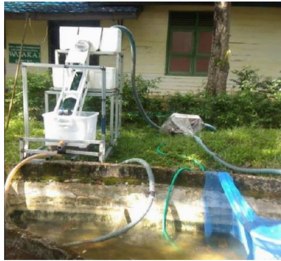
Figure 4. MHP Prototype with Archimedes Screw Turbine
