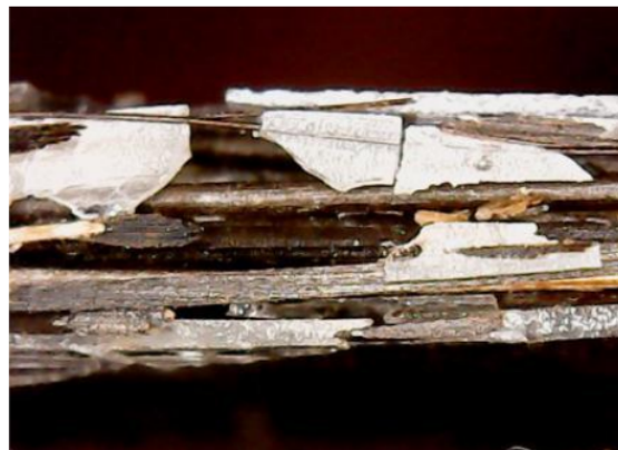
Figure 5. Macro photo of composite fracture (composite composition 40:60)
