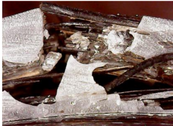
Figure 6. Macro photo of composite fracture (composite composition 50:50)
