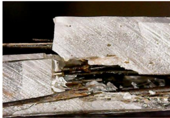
Figure 4. Macro photo of composite fracture (composite composition 30:70)
