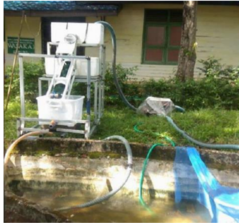
Figure 4. MHP Prototype with Archimedes Screw Turbine
