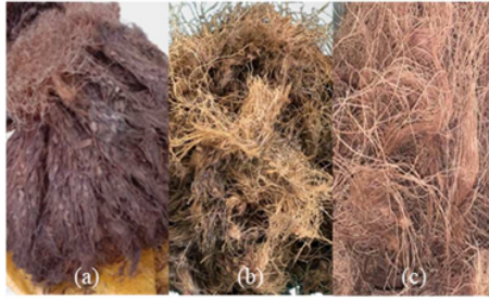
Fig. 1 Fiber preparation from the row material of an empty fruit bunch to the fine fiber (a) oil palm empty fruit bunch (OPEFB), (b) empty fruit bunch shredded fiber, and (c) final fiber as used.
