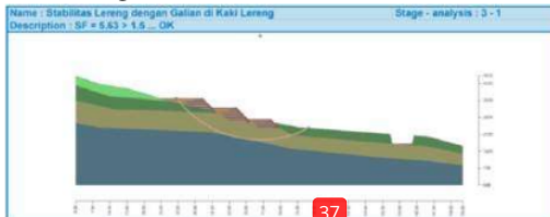
Figure 4. 10 Results of Slope Stability Analysis with Excavations at the Foot of the Slope
