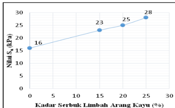
Gambar 3.7 Hubungan antara Nilai S_u vs prosentase arang
