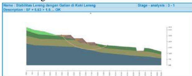
Figure 4. 10 Results of Slope Stability Analysis with Excavations at the Foot of the Slope
