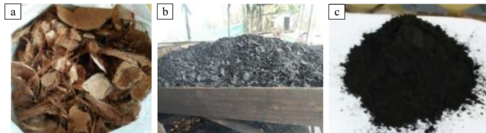
Figure 1. (a) coconut shell; (b) burnt coconut shell; (c) sieved coconut shell ash (CSA)
