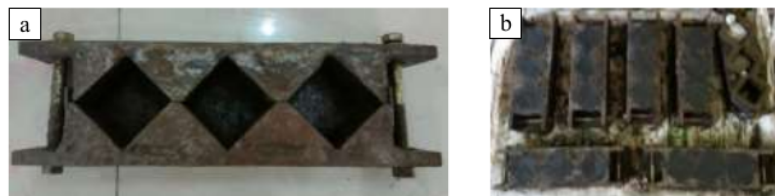
Figure 2. (a) mortar mold cube of 5 \times 5 \times 5cm; (b) after casting
