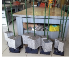
FIGURE 3. The pull-out specimens prepared before the test.
