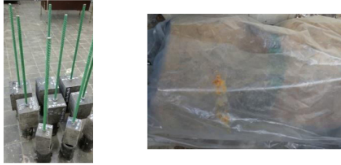
Fig. 2. (a) Pull-out specimens after demolding; (b) Curing pull-out specimens
