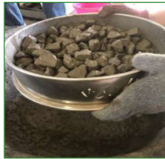
Figure 3. The coarse aggregate was retained on a sieve.
