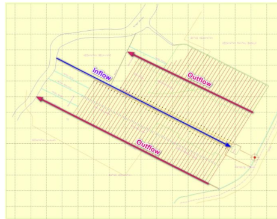
Figure 2. One-Way Flow System
