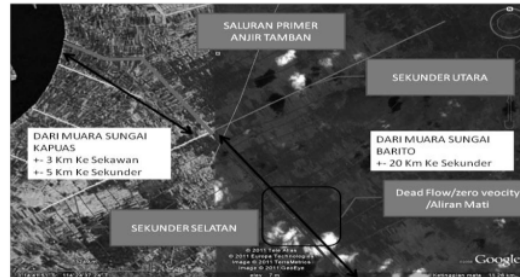
Fig. 2 Layout of Macro Water System
