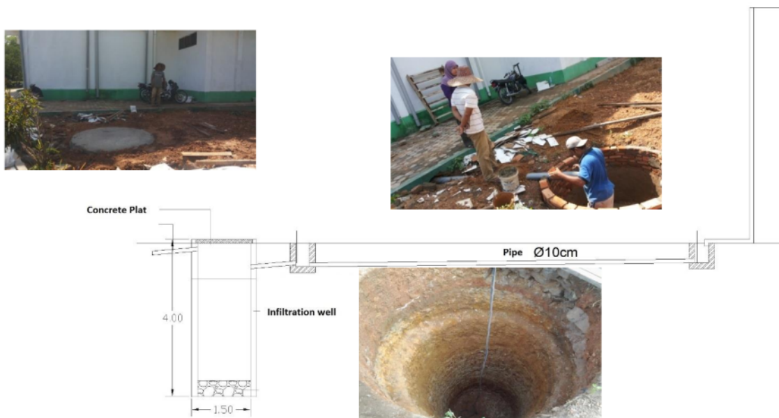
Figure 3. Infiltration well detail
