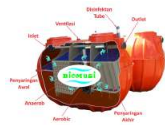
Gambar 17. Cutaway Septic Tank Biofill Sumber: www.biomusi.com
