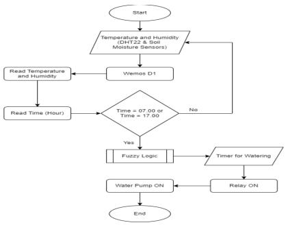
Figure 3. System Workflow
