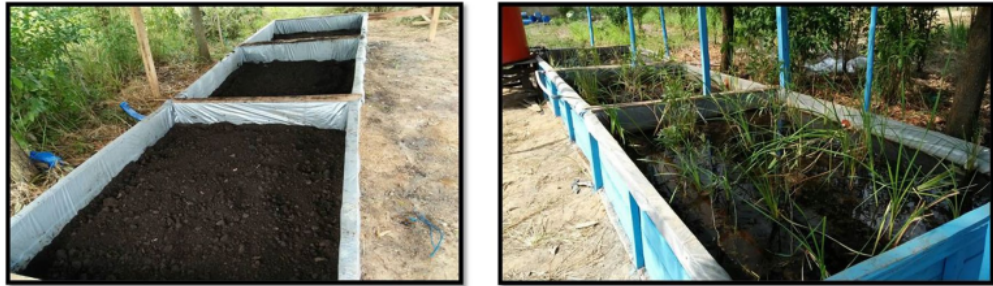
Figure 4. The picture of experimental box (reactor) for laboratory simulation to treat the AMD to change not comply parameter at inlet to be comply at outlet (personal documentation).
