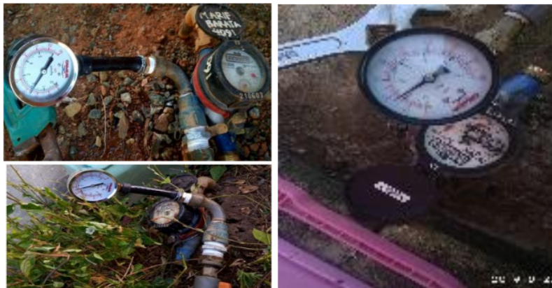
Figure 2. Calibration at several junctions
