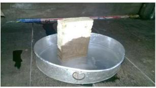
Figure 6. Soaking Bricks for Salt Crystals Observation
