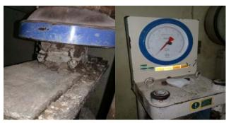
Figure 5. The Bricks Compressive Strength Test
