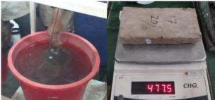
Figure 7. The Brick Apparent Density Test
