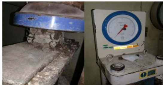
Figure 5. The Bricks Compressive Strength Test
