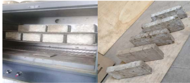
Figure 3. The Brick Visibility Test in Oven-Dry Condition
