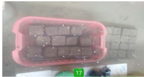
Figure 8. The Bricks Water Absorption Test
