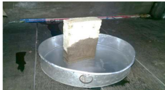
Figure 6. Soaking Bricks for Salt Crystals Observation
