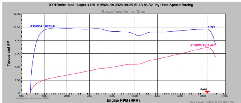
Gambar 4. Performance mesin tanpa adsorben
