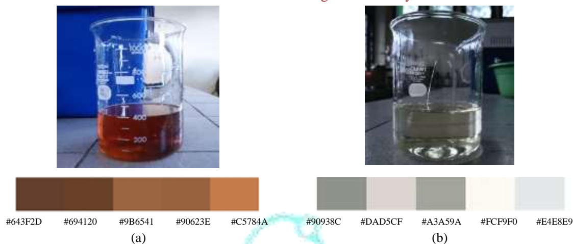
Figure 3. Color comparison between crude glycerol and purified glycerol using a color palette
