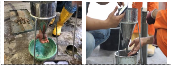
Figure 5. Flow cone test.
