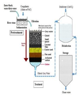
**Figure 2.** Water Purification Methods with Coagulation, Sedimentation, Filtration, Adsorption, and Chemical Disinfection (Syahmani, Kusasi, et al., 2021)
