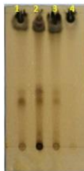
Picture 2. Polyphenols TLC analysis of ethanol extract of leaves 1 , stem bark 2 , wood 3 and pericarp 4 .
